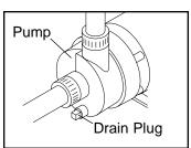
Remove the drain plug from the pump. Tip the spa jet unit slightly until all the water has drained from the pump. Replace the drain plug.
